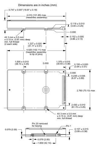
Figure 2. Mounting dimensions for the ST9655 family drives
