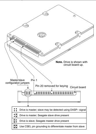
Figure 1. ATA interface connector and master/slave configuration jumpers
