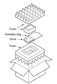
Figure 3. Seagate 2.5-inch drive and approved packing materials
